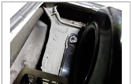
Remove heater box lid-check bulkhead
