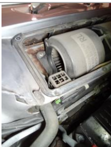
Remove heater box lid-check bulkhead
